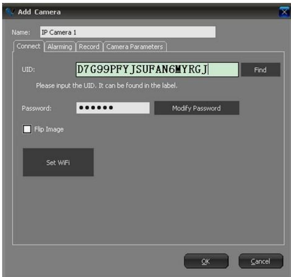
press "Set WIFI",to set a Camera to wirelessly connect to Router.
