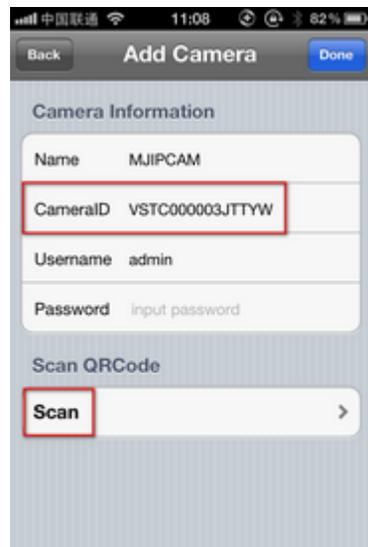
Point iPhone camera towards the UID (The UID can be found on the bottom of the IP camera or the warranty card). After a “beep” sound, the UID is scanned successfully. Also you can click “search” to add cameras in the LAN, or manually " Add camera", to input the camera's UID and password. The default password is blank.
