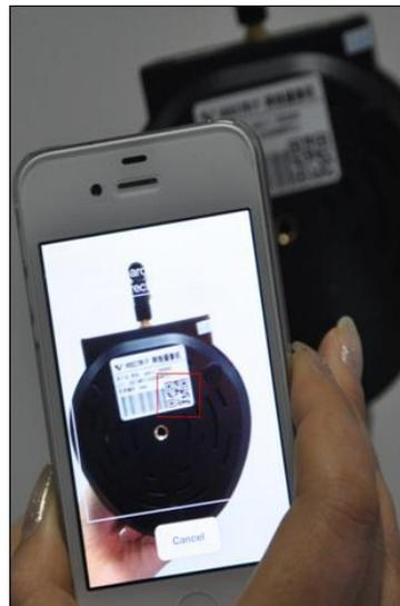
Use mobile to scan QR code(can be seen on the bottom on the IP camera or printed on the label). When mobile scans the code successfully, there will be a string displayed on the Textbox.
